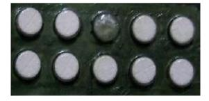
Figure 7 Tablet packet with missing tablet
